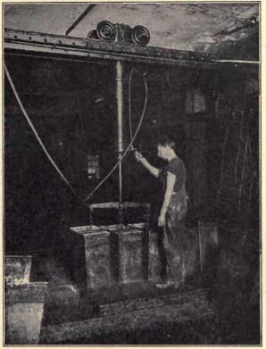
Lifting Cans by Compressed Air Lift from Freezing Tank.
